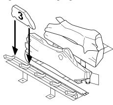
Figure 53 - Installing Log No. 3
